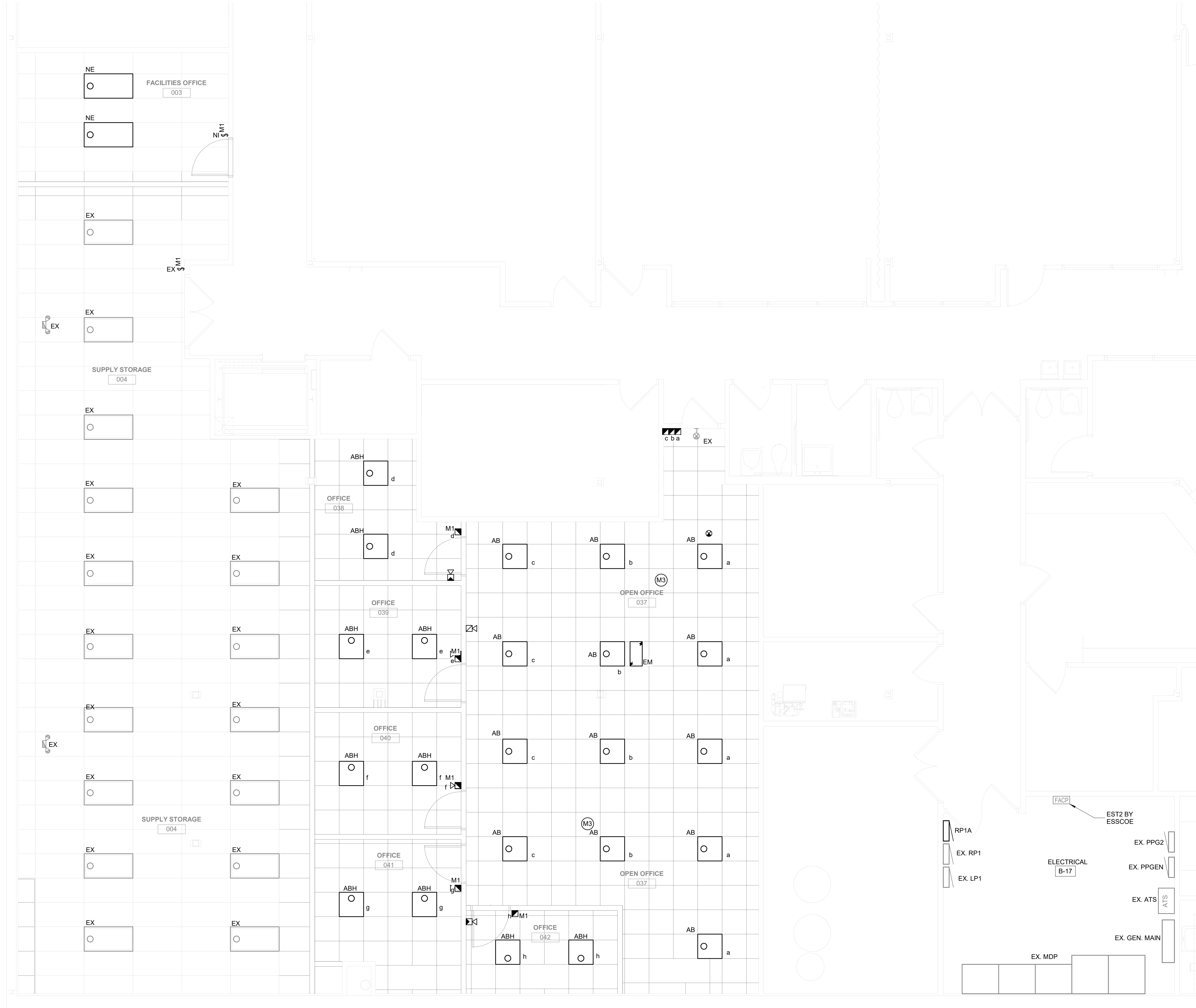
1 ELECTRICAL LIGHTING FLOOR PLAN 1/4" = 1'-0"
